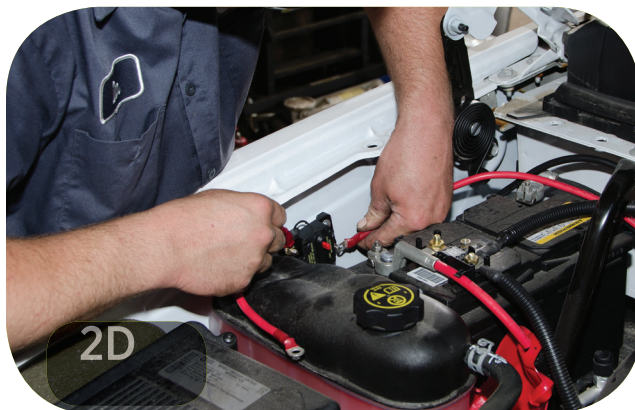
2D Mount the 50 amp breaker very close to the positive battery terminal. (Connection to the breaker is shown in Step 1D.)
