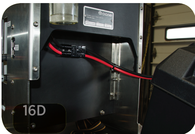
Connect machine's onboard battery to the Promist's power plug.
